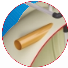
Main Inlet 2.0, 2.5 and 3.0 metre invert depths.
